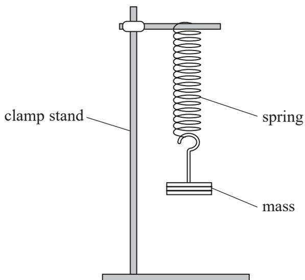
She set the mass into vertical oscillations by displacing it a small distance from its equilibrium position. The spring obeys Hooke's law.
